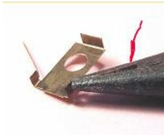
Taper the straight wing by holding the wing with pliers.
