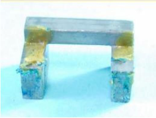
Some of the weights are glued to the tender shell. Liberally apply MEK or laquer thinner at the arrows on both sides and use an knife and screwdriver to loosen the weight.
