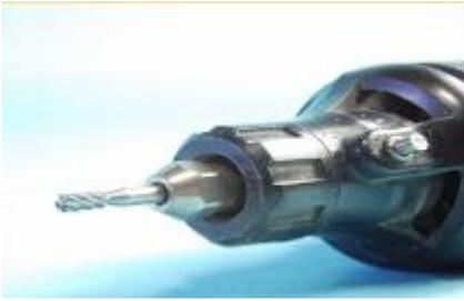
**A motor tool with a 1/8" diameter burr makes the conversion easier. I find this the most controllable size.**
