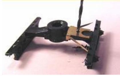
Place the spring on the sideframe and drill and tap for a #00-90 screw.
