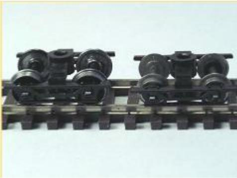
Kadee #5 centering springs for electrical pickups and 28" wheels are used in the conversion. I like the Kadee wheels because they have recessed back and look more prototypical and are readily available cheap.
