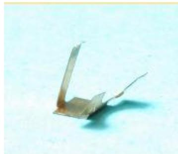
Cut the original wipers in half and bend them as shown. Slide them under the truck pickups. Cut about a 1/16" off of the wiper blade.
