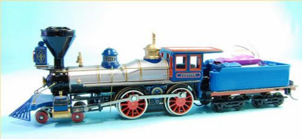
This is our "beta" locomotive, excuse the disrupted cross heads and other cosmetic problems. The loco has a "daylighted" cab, Soundtraxx Tsunami sound, prototypical spacing between loco-tender, bigger tender wheels and will crawl along.
