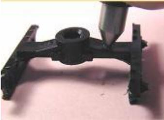
Use the truck reamer to break the edge of the tapped hole to make the insertion of the screw easier.
